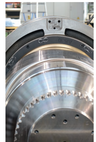
An eccentric shaft with oil drainage rings
