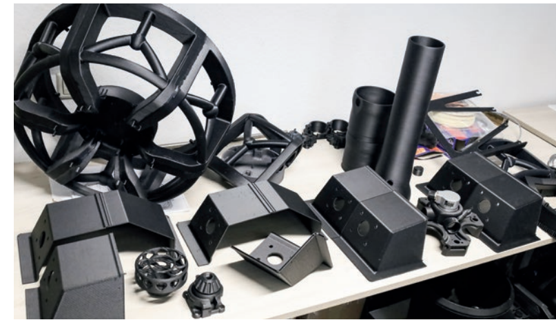
Various components produced by Tec-Farm, including a mount for the main motor encoder (top left)
