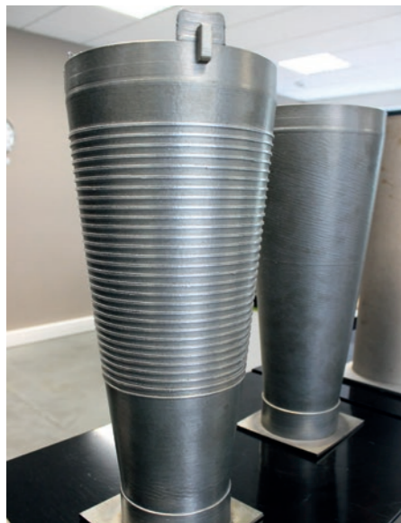
Photo on top: Test components for engine nozzles for the aviation sector in Inconel 625.
