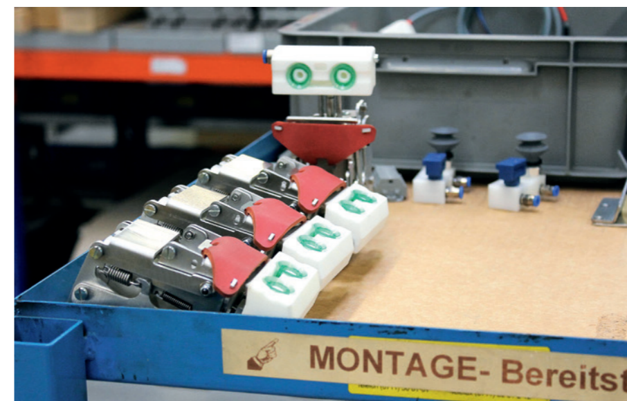
Photos above and below: Components for printing equipment. The suction unit was not only produced using additive techniques, but also optimized in the process.
